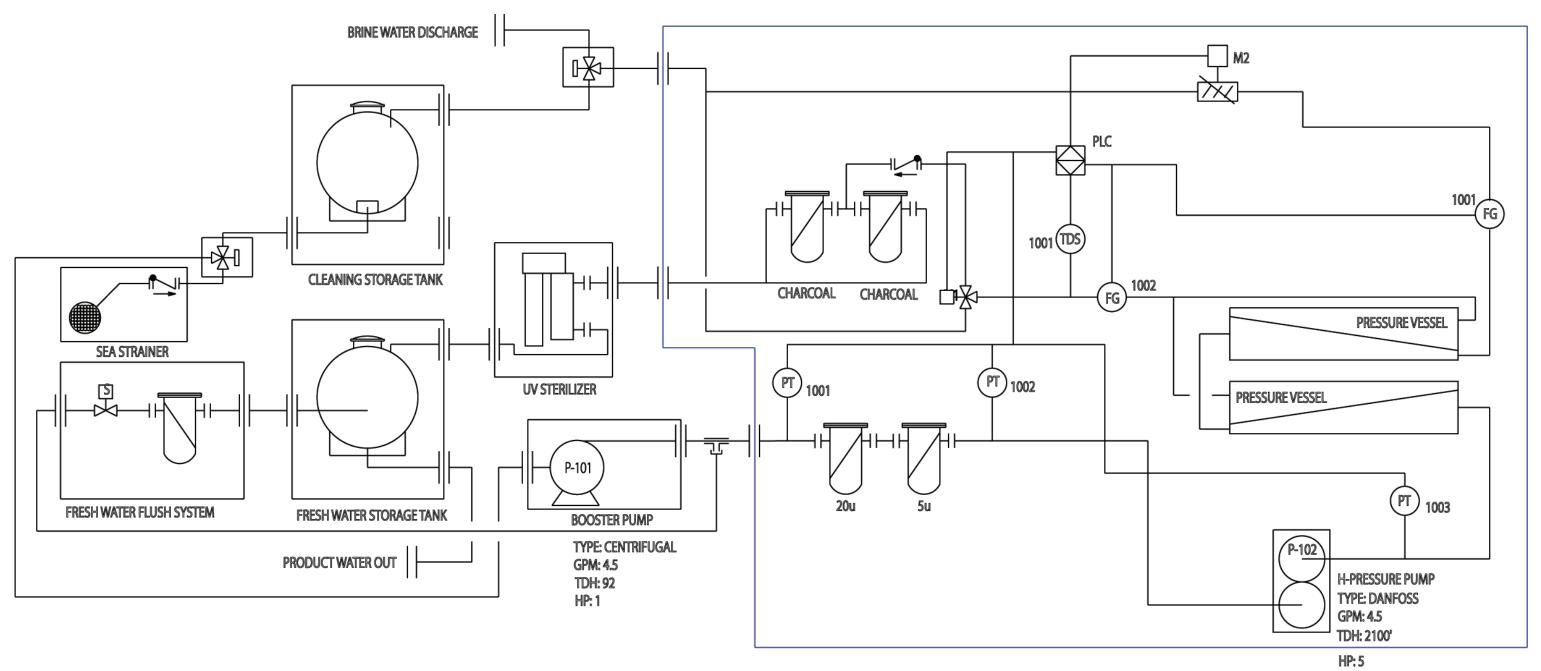
PT-Pressure Transducer PI-Pressure Indicator M-Meter FG-Flow Gauge TDS-TDS Meter P-Pump PLC-Program Logic Controller
