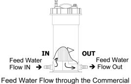
Feed Water Flow through the Commercial Prefilter Element is from the OUTSIDE of the Element to the INSIDE CENTER of the Element
