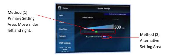
The Salinity value range is 150PPM to 999PPM. Once the value is entered, the slider position, and the current setting value will update appropriately.
