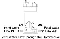
Prefilter Element is from the OUTSIDE of the Element to the INSIDE CENTER of the Element
