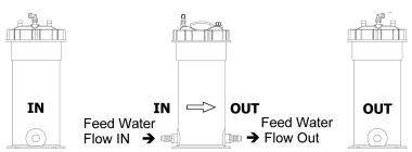
Commercial Prefilter is plumbed as per the raised arrows and markings IN and OUT
