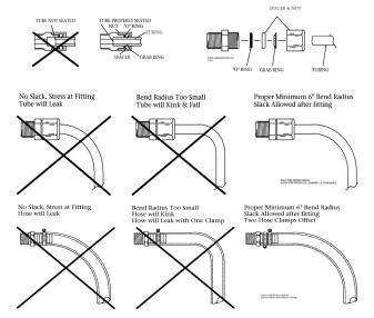
Figure 5c - Always allow slack in all tube and hose lines.
