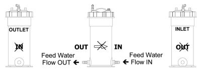
Oil/Water Separator utilizes the same housing as the Commercial Prefilter, however it is plumbed OPPOSITE of the Commercial Prefilter and OPPOSITE of the raised arrows and markings IN and OUT Separate Labels are placed on the Oil/Water Separator indicating correct INLET and OUTLET
