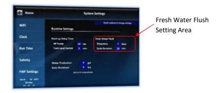
7. Press Fresh Water Flush Frequency to change the default number of days between fresh water flushing.
