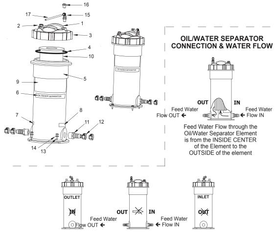
Oil/Water Separator utilizes the same housing as the Commercial Prefilter, however it is plumbed OPPOSITE of the Commercial Prefilter and OPPOSITE of the raised arrows and markings IN and OUT Separate Labels are placed on the Oil/Water Separator indicating correct INLET and OUTLET
