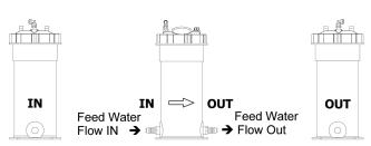
Commercial Prefilter is plumbed as per the raised arrows and markings IN and OUT
