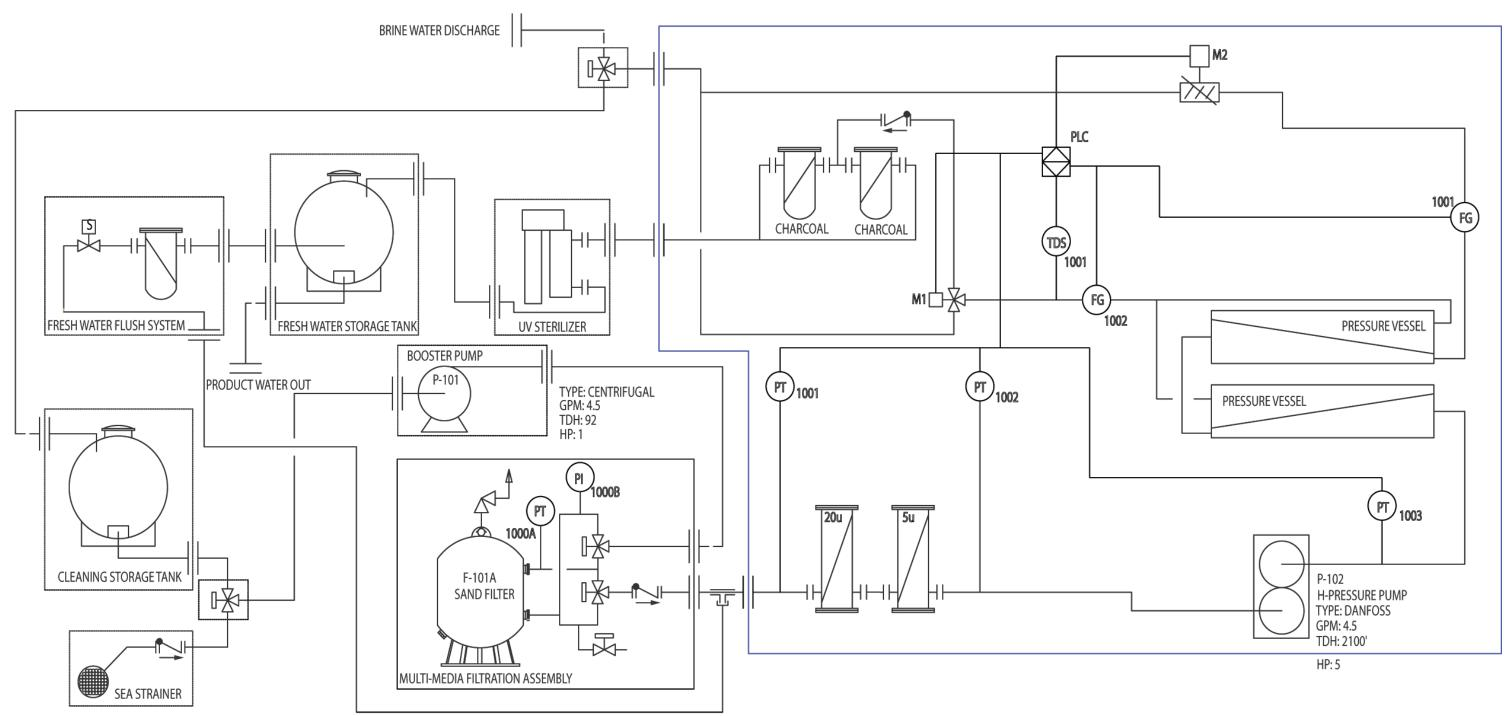
PT-Pressure Transducer PI-Pressure Indicator M-Meter FG-Flow Gauge TDS-TDS Meter P-Pump PLC-Program Logic Controller
